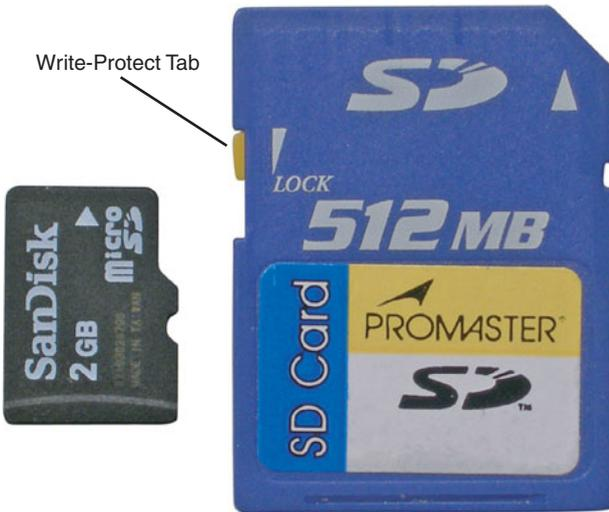
FIGURE 6.7 A typical microSD card (left) and a standard SD card (right)
