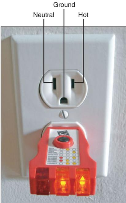
FIGURE 5.1 A common receptacle tester and labeled receptacle
