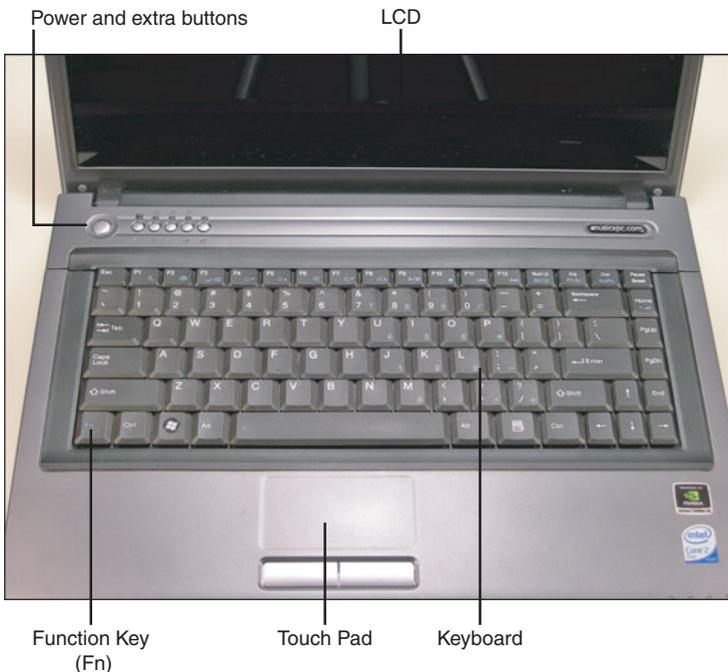
FIGURE 11.1 A typical laptop's main components
