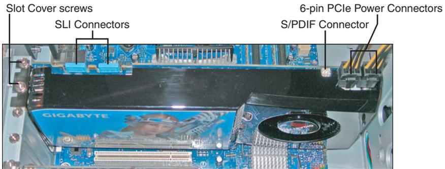
FIGURE 12.4 An installed PCIe GTX 260 video card
