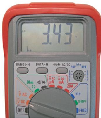
FIGURE 5.11 Testing the 3.3 volt wire with a multimeter set to volts DC
