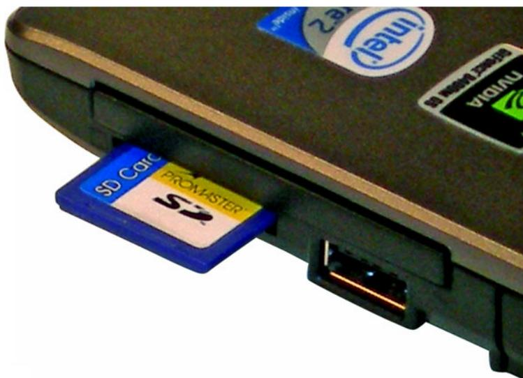
FIGURE 6.8 A standard SD card inserted in a laptop's Memory Card Reader.
